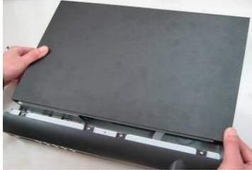
7. Put the cover in accordance with the clip and then place the upper cover back.
