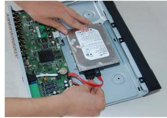
6. Connect the HDD cable and power cable.
