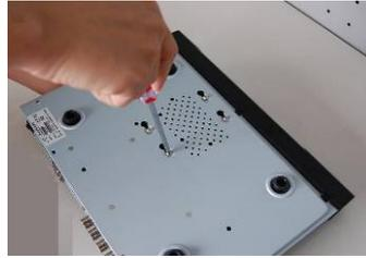
5. Fix the HDD firmly.
