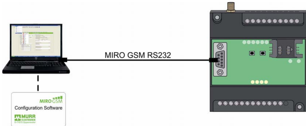
Fig. 4: Connecting a PC or notebook with RS232 interface
