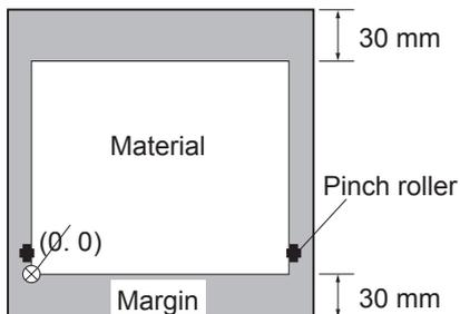
After length in the direction of material feed is detected, movement 30 mm (1-3/16 in.) back from the front edge of the material is performed, and the origin point is set near the left pinch roller.
