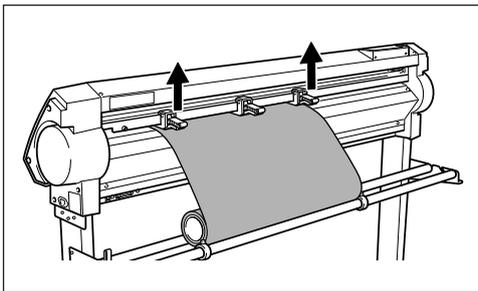
While keeping the material stretched taut, raise the sheet loading levers to secure the material in place.
