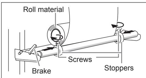
**Position the stoppers so that they lightly touch the edges of the roll and secure in place by tightening the screws.**
