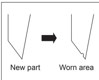
If any of the following occurs, it means the blade has reached the end of its useful life. Replace with a new blade.
