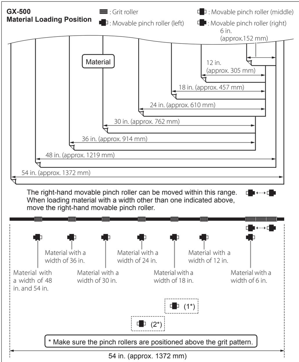
(1\*) Position of the pinch roller (middle) when using material with a width of 30 in. or 36 in.
