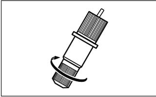
If material debris is adhering to the inner surface of the cap for the blade holder, loosen and remove the cap, then remove the material debris. If corners and curves are not cut attractively, or if cutting is discontinuous, clean the blade holder cap.
