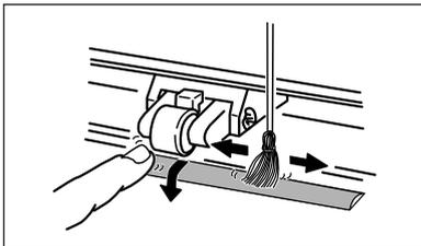
With the sheet loading levers lowered and the pinch rollers raised, use a commercially available brush to remove dust and other detritus. Brush horizontally while rotating the grit rollers.
