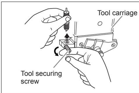
Loosen the tool securing screw, and remove the blade holder from the tool carriage.
