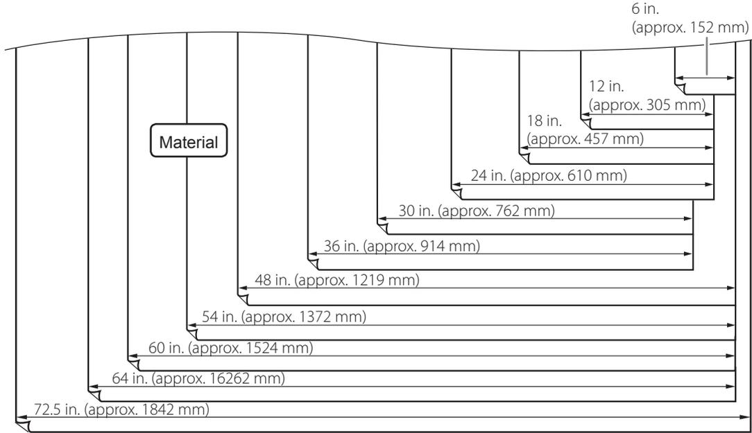
The right-hand movable pinch roller can be moved within this range. When loading material with a width other than one indicated above, move the right-hand movable pinch roller.
