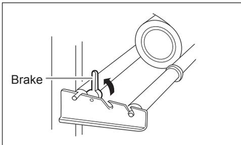
Place the roll material on the shaft and engage the brake for the shaft.
