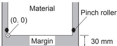
Set the origin point at a location having a margin of 30 mm (1-3/16 in.) from the front edge of the material.
