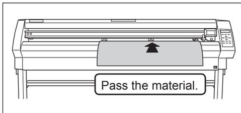
Lower the sheet loading levers and pass the material between the pinch rollers and the grit rollers.
