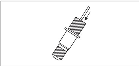
Insert the pin into the blade holder.
