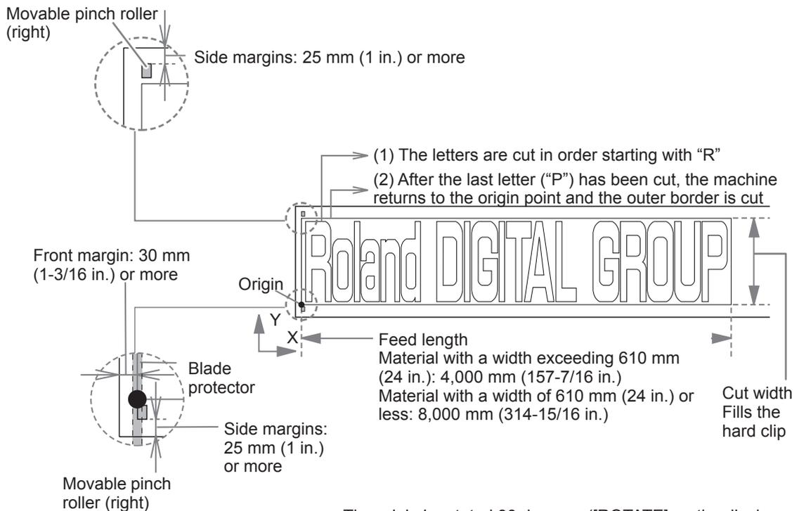
The origin is rotated 90 degrees ([ROTATE] on the display menu is set to [90deg]).
