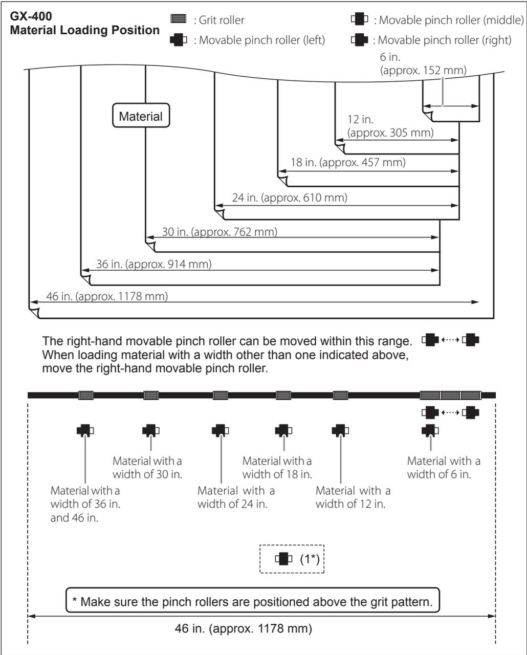
(1\*) Position of the pinch roller (middle) when using material with a width of 30 in. or more.
