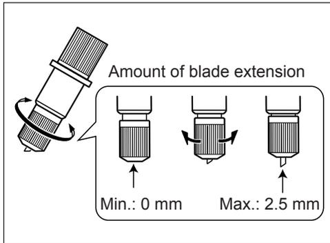
Each indicator tick corresponds to 0.1 mm, and adjustment for 0.5 mm can be made by rotating the cap one full turn.
