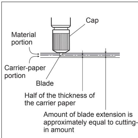
Turn the cap portion to adjust the amount of blade extension, which is approximately equal to the cutting-in amount. Setting the blade force slightly higher than normal achieves a stable cutting-in amount.
