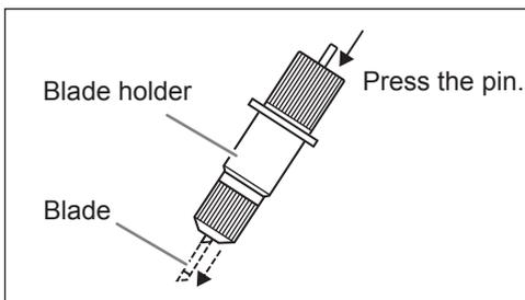
Press the pin and remove the blade from the blade holder.
