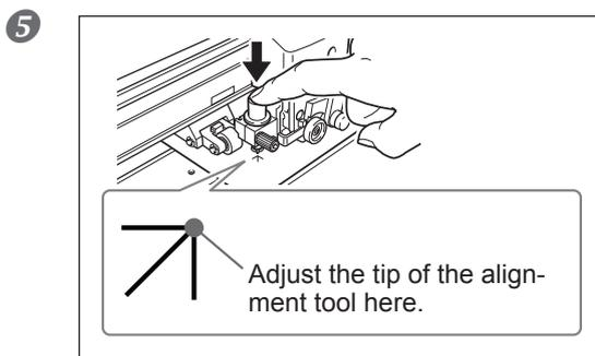
**In the same way as for mark 1, align the tip of the alignment tool with the crop mark.**
