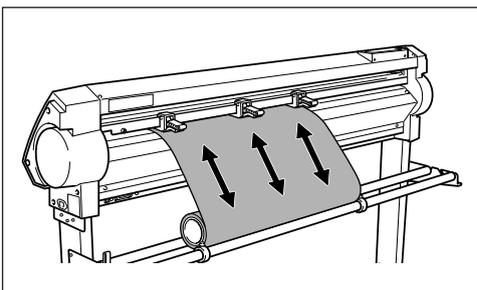
Pull out the material from the roll and pass it through the unit.
