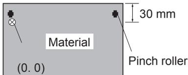
Set the origin point at a location having a margin of 30 mm (1-3/16 in.) from the trailing edge of the material. When in this state, the cutting area is zero.
