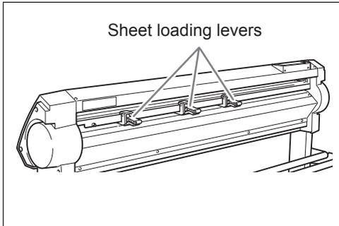
Lower the sheet loading levers to raise the pinch rollers.
