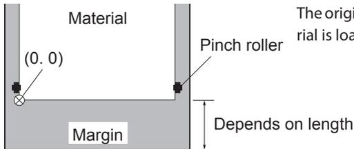
The origin point is set at the location where the material is loaded, near the left pinch roller.
