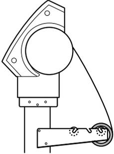
Performing high-speed cutting when only a little roll material remains may cause the roll to fall off the shafts. If this happens, it may help to pass the shaft through the roll.
