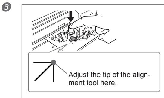
Press to align the tip of the alignment tool with the crop mark.
