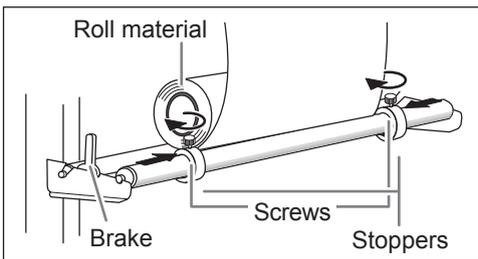
Position the stoppers so that they lightly touch the edges of the roll, and secure in place by tightening the screws.
