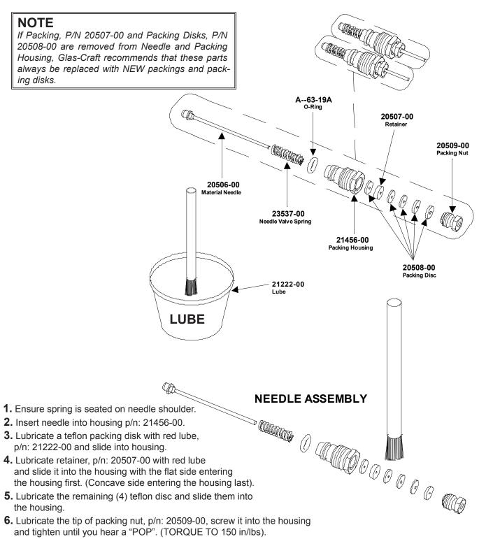
7. Instal and lube o-ring, p/n: A-63-19A and Re-install needle assembly.
