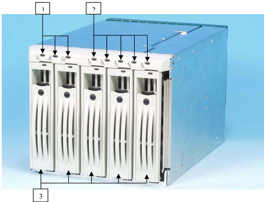
1. Voltage level, Temperature, Fan Indicator
