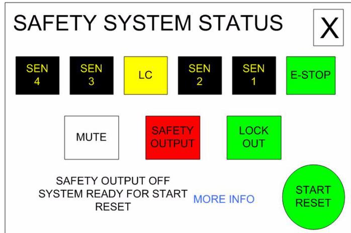
13. Press START RESET for three seconds and release.
