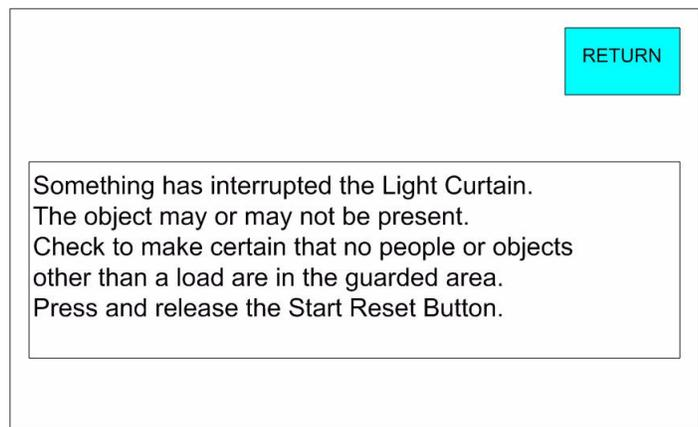
12. Remove the object interrupting the light curtain.
