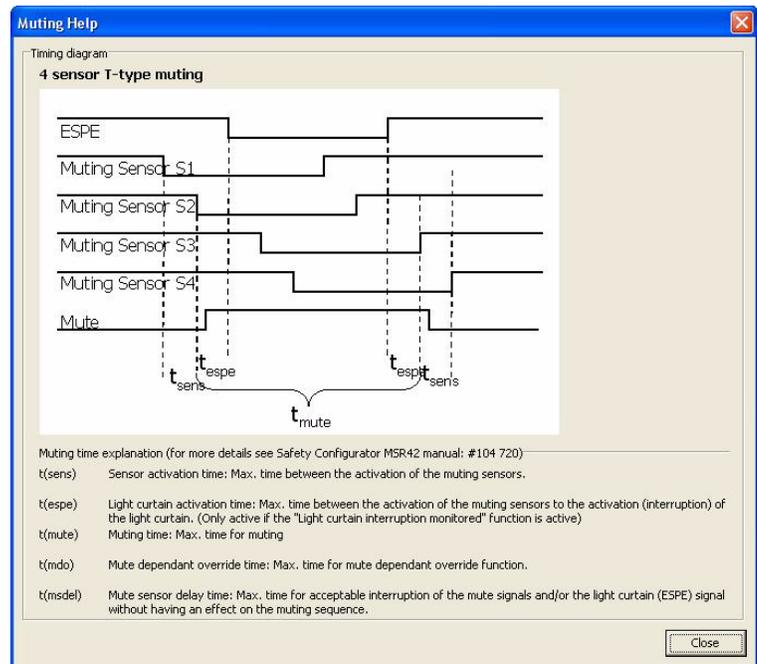
The Muting Help dialog box also provides definitions for the  $t(\text{sens})$ ,  $t(\text{espe})$ ,  $t(\text{mute})$ ,  $t(\text{mdo})$ , and  $t(\text{msdel})$  times, which you can configure on the 4 sensor T-type dialog box. A load that exceeds any of these configured times as it moves across the conveyor causes a muting error, which results in the light curtain not being muted. A load entering the light curtain sensing field during a muting error triggers a safe stop.
