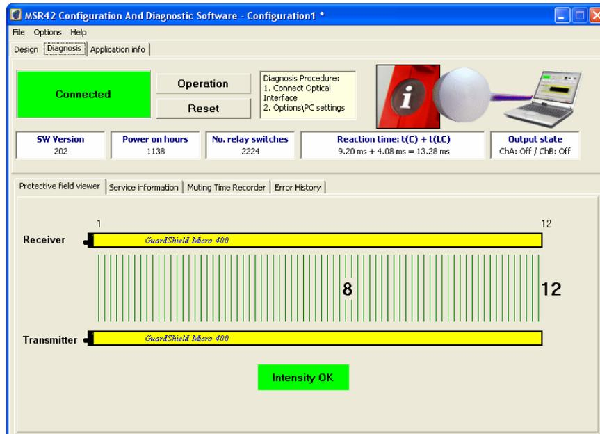
This screen lets you monitor the status of the light curtain when a computer is attached to the MSR42 relay via the Optical Interface. It has other helpful diagnostic features that are described in the MSR42 Safety Base Module Operation Manual, publication [440R-IN017](#), and the Configuration Tool for MSR42, GS Micro 400 and Safe 2/4 Light Curtains Software Description document, available on the CD that ships with the Optical Interface tool.
