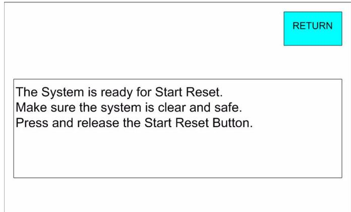
The system should start running. Note that the START RESET button is green only when the system is ready for a Start Reset. It is no longer green once the system is running.
