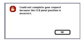
The CCD pixel position value may become corrupted as the result of a power surge or failure. If this occurs, you must find the correct value and enter it as described in the following procedures before starting a run.
