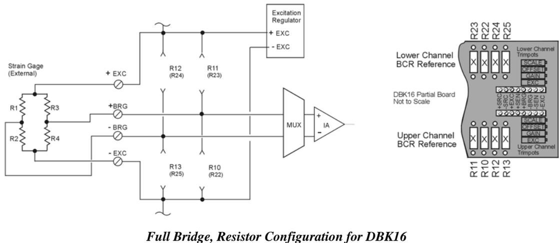
The full bridge configuration makes use of all four elements of the strain gage. When using a full bridge external strain gage (all four elements), the following applies to the DBK16 on board resistor configuration:
