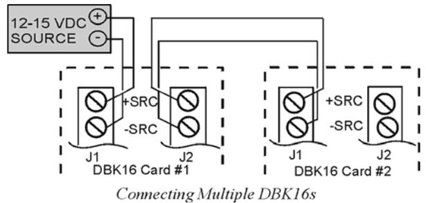
The user-supplied excitation source is attached to a voltage regulator in the DBK16 circuitry. This regulator provides the excitation to the actual transducer (there is a separate regulator for each transducer, hence two regulators per DBK16). Each regulator has a maximum current of 50 mA. The maximum amount of excitation that can be provided by the DBK16 excitation regulator is represented by the following equation:
