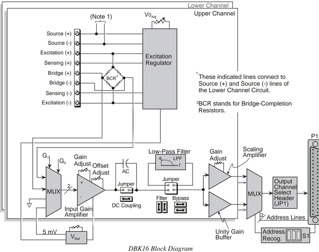
A wide-range excitation regulator is adjustable from 1.5 to 10.5 VDC with a current limit of 50 mA. The DBK16 requires a 12 to 15 VDC external excitation voltage that can be supplied from the DBK30A battery module or other user-supplied source.
