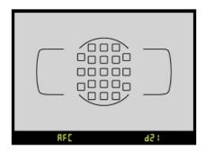
In this mode there are a maximum of twenty-one sensors that are active. The center sensor is the selected sensor for the initial point of focus and the other twenty are for assist. The functionality is very similar to the d9 functionality just discussed.
