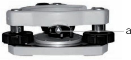
1. Turn the screw on knob **a** outward using flat screw driver until it no more limits position.
