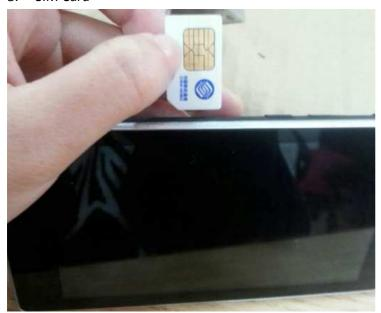
SIM card can be inserted into the host to achieve some phone functions, such as SMS, call, etc. SIM card supports 850/1900 and 900/1800, no supports CMDD.
