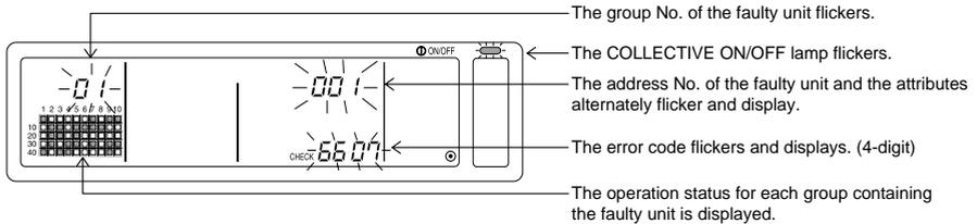
1. If an error occurs while the [Collective Setting/Monitor Screen] is displayed, the details of the error for the group containing the first problem will appear.
