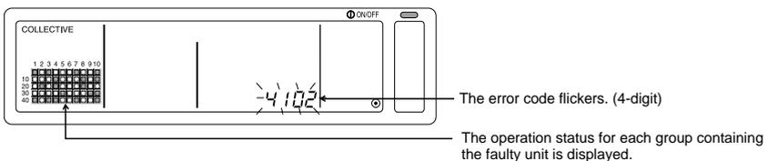
1. If an error occurs while the [Collective Setting/Monitor Screen] is displayed, the details of the error for the group containing the first problem will appear.
