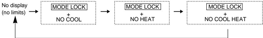
When “NO COOL” is selected : The cooling, dry or automatic modes cannot be selected with the (MODE) switch.
