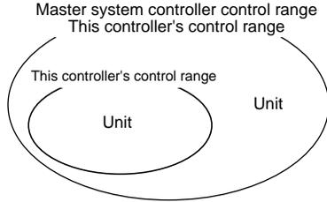
When this controller is controlled by another system controller. This controller is set as the slave system controller. In this case, the group is not set with this controller.
