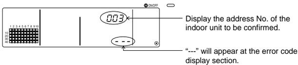
Press the **MODE LOCK** switch in the above state.
