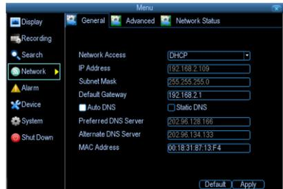
**IP Address:** Just as houses and businesses need to have an address which identifies their location on the road network, so too do computers and other devices need addresses (called IP ADDRESSES) to identify their position on the electronic network. The DVR uses IPv4 addressing, which consists of four groups of numbers between 0 and 255, separated by periods.
