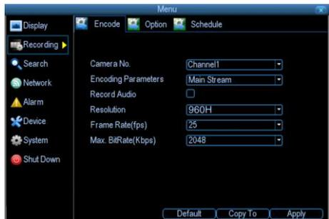
**Encoding Parameters** (advanced user option): Whether you’re editing the parameters for the mainstream or the sub stream.
