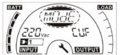
Step 6: “CVF” flickering after pressing the “Select” button again. Press the “Enter” button to make sure to change the mode. Short touch “Enter” button to exit setting mode.
