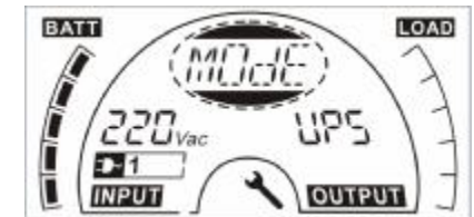
Step 4: “MOdE” after pressing the “Select” button, press the “Enter” button to set mode, then “UPS” flickering;
