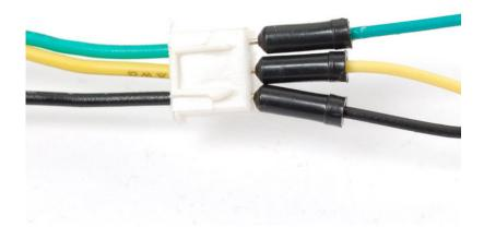
At the Arduino end, the **green** wire connects to **digital pin 5**, **yellow** goes to **digital pin 6** and **black** to any of the **GND** pins. You can change the digital pins later, but to match the example code, stick to this for now!
