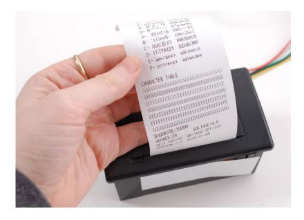
If you don't get a printout, check that the paper is inserted correctly and not binding, that the power is correctly wired, power supply is plugged in, etc. Then try again, holding down the top button when connecting power.
