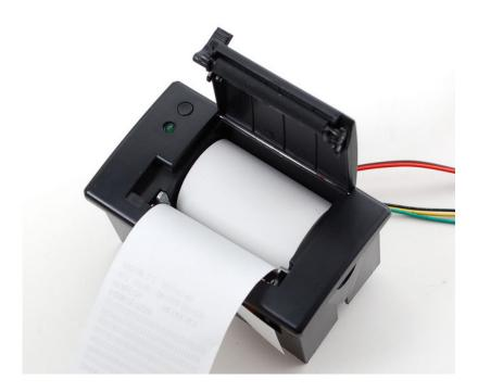
As previously described, power the printer using a 5V to 9V 1.5A or higher power supply, such as wiring up a 2.1mm DC power jack:
