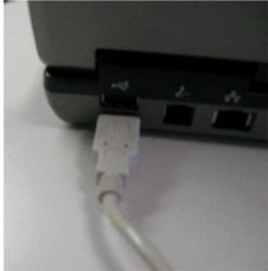
USB cord - connects from the back of the board to any USB port (it must be plugged into the same port every time)
