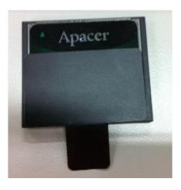
Step 3 Insert the CF card to the CF card slot, then finding the CF cover from the system package and screw it.
