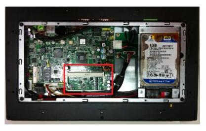
Step 4 Insert the DRAM to the DIMM socket, and then push it down firmly until it is clipped by the socket.
