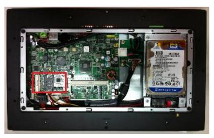
Step 2 Insert the wireless LAN card to the slot. Push it down firmly until it is clipped by the slot.
