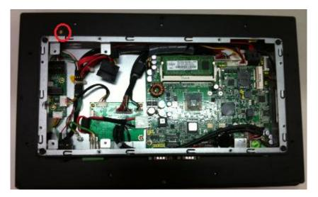
Step 5 Install the antenna on the antenna connector.
