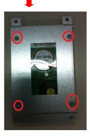
Step 3 Plug the cables to connectors and screw the HDD tray on the bracket. Installation completes.
