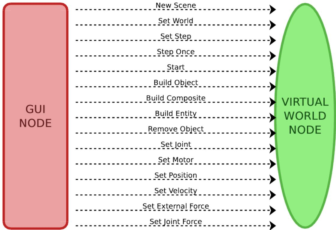
Figure 3.6: Services called from the *GUI* and replied by *VirtualWorld*.
