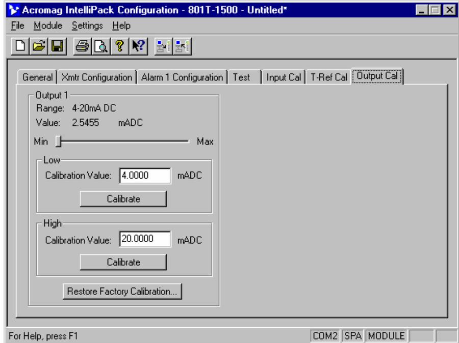
For best results, you will need a precision milliammeter or voltmeter capable of resolving the selected output current or voltage range and at least as accurate as the module itself. A properly calibrated output stage will indicate a screen "Value:" matching the value measured via the meter.
