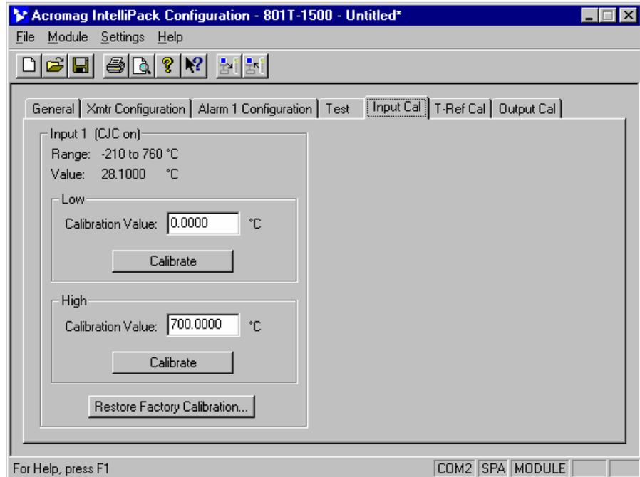
If you make a mistake, or your calibration appears in error, you can use the "Restore Factory Calibration" button to restore a module's original factory input calibration (only the input calibration will be affected).
