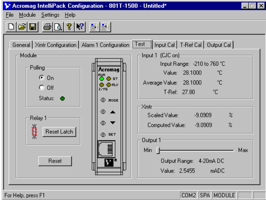
This control will temporarily override input control of the output, allowing you to verify output operation.
