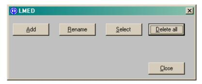
**Add:** Allows you to enter the number of DGID readers on the network. The quantity can be modified at any time.
