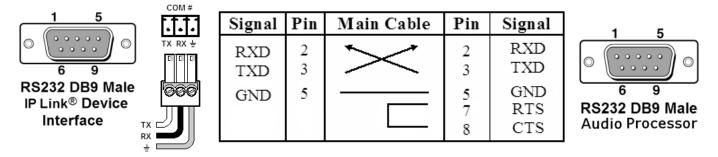
Note: Captive screw connector may also be used as a serial connection.
