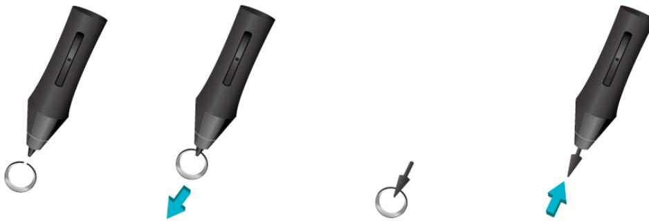
B: Push the pen tip into the digital pen, Make sure fit it up to the end properly.
