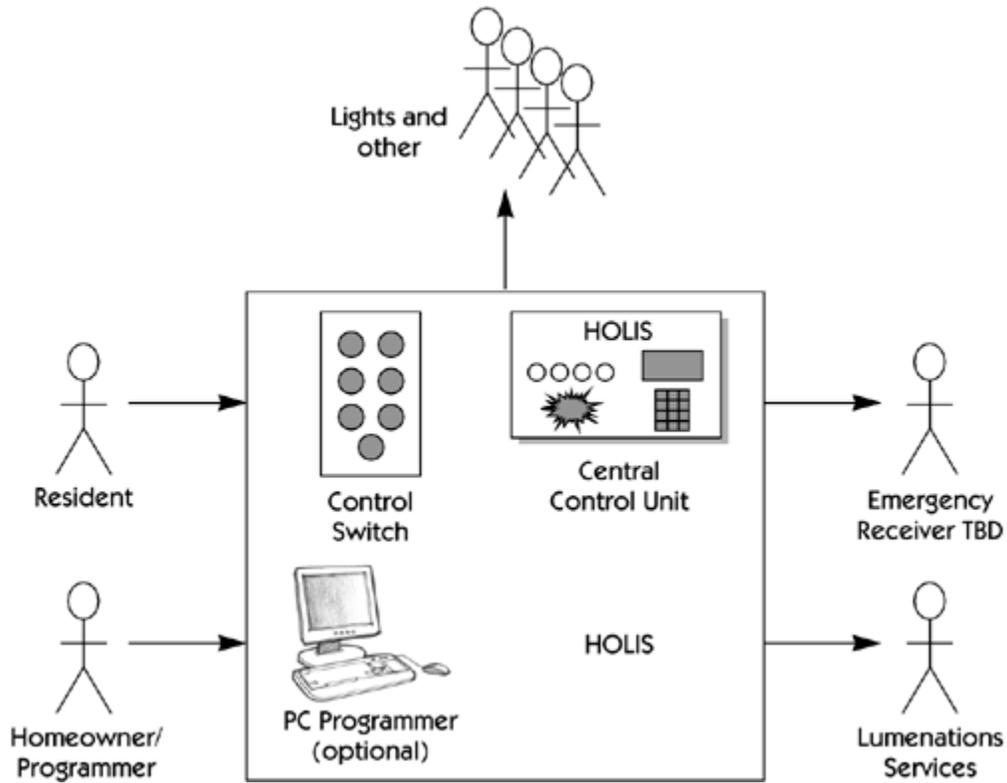
Figure A-3. Control Switch subsystem with actors
