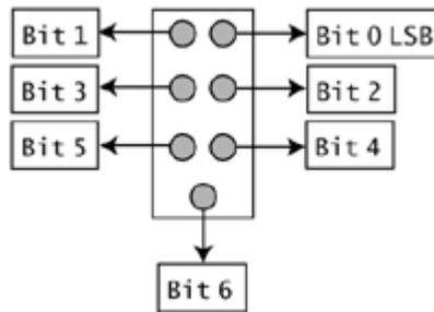
SR4.3. **Data**, each bit corresponding to a specific button on the key switch.
