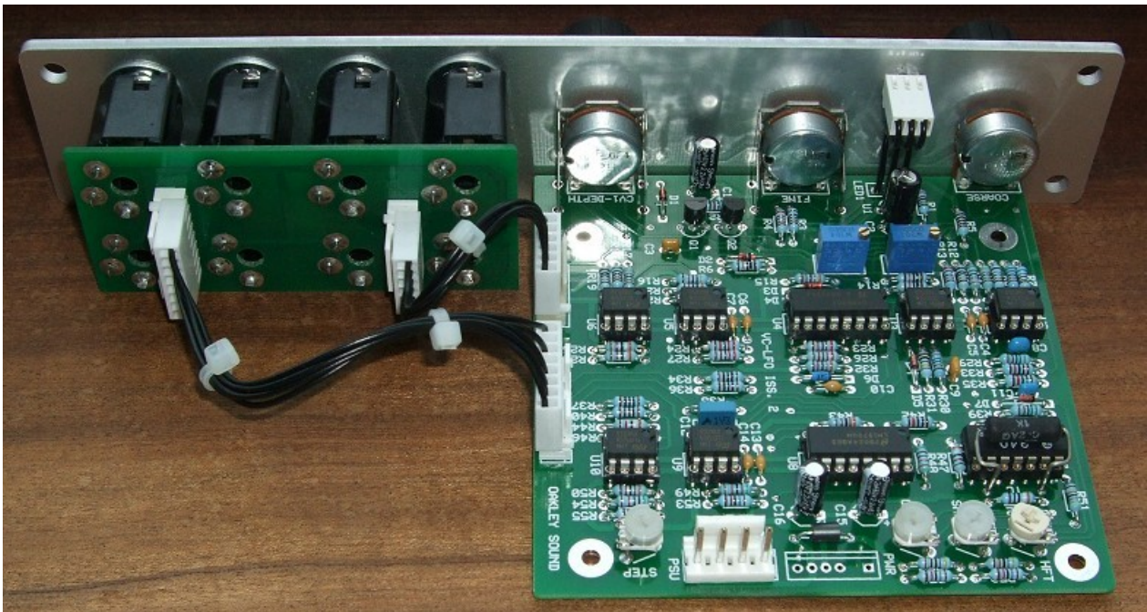
The issue 3 PCB mounted behind a natural finish panel. Note the use of the optional Sock8 socket board to facilitate the wiring up of all those sockets.
