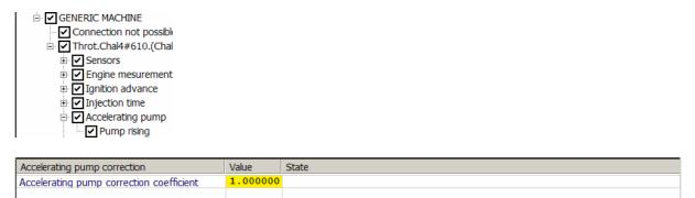
Higher is this coefficient, higher is the acceleration pump, which means that the engine is richer on the accelerations.
