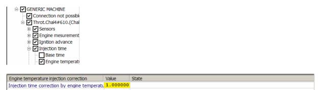
Higher is this coefficient, higher is the engine temperature correction, which means richer is the engine at cold state.
