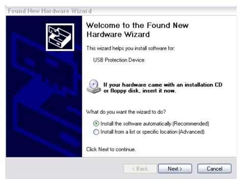
Select "Install the Software Automatically (recommended)", and click "Next". Windows will locate the driver and install it.
