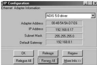
All Ethernet adapter information is shown in this window. Check if you get an IP address like 192.168.8.x and the default gateway is 192.168.8.1.
