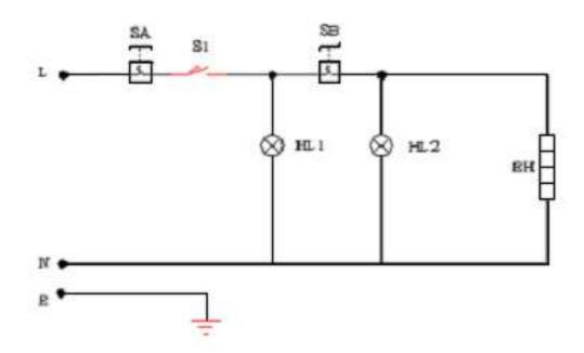
S1—MICRO-SWITCH SB—TEMPERATURE CONTROLLER HL1—POWER INDICATOR
