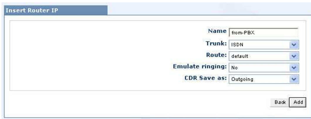
Figure 6.11 – Router IP configuration
