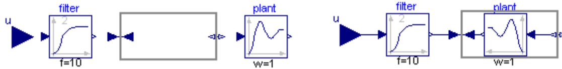
Figure 19.8: Definition of inverse model in Modelica (left part: the 4 basic components; right part: the 4 basic components connected together).
