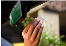
2. When the mounting area is dry, carefully peel off the adhesive tape from the clip and affix the unit on the front windshield. Ensure that the tag is positioned correctly as it is not easily removable.
