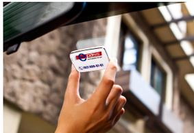
3. Press the tag onto the windshield for a few seconds to ensure a strong bond.
