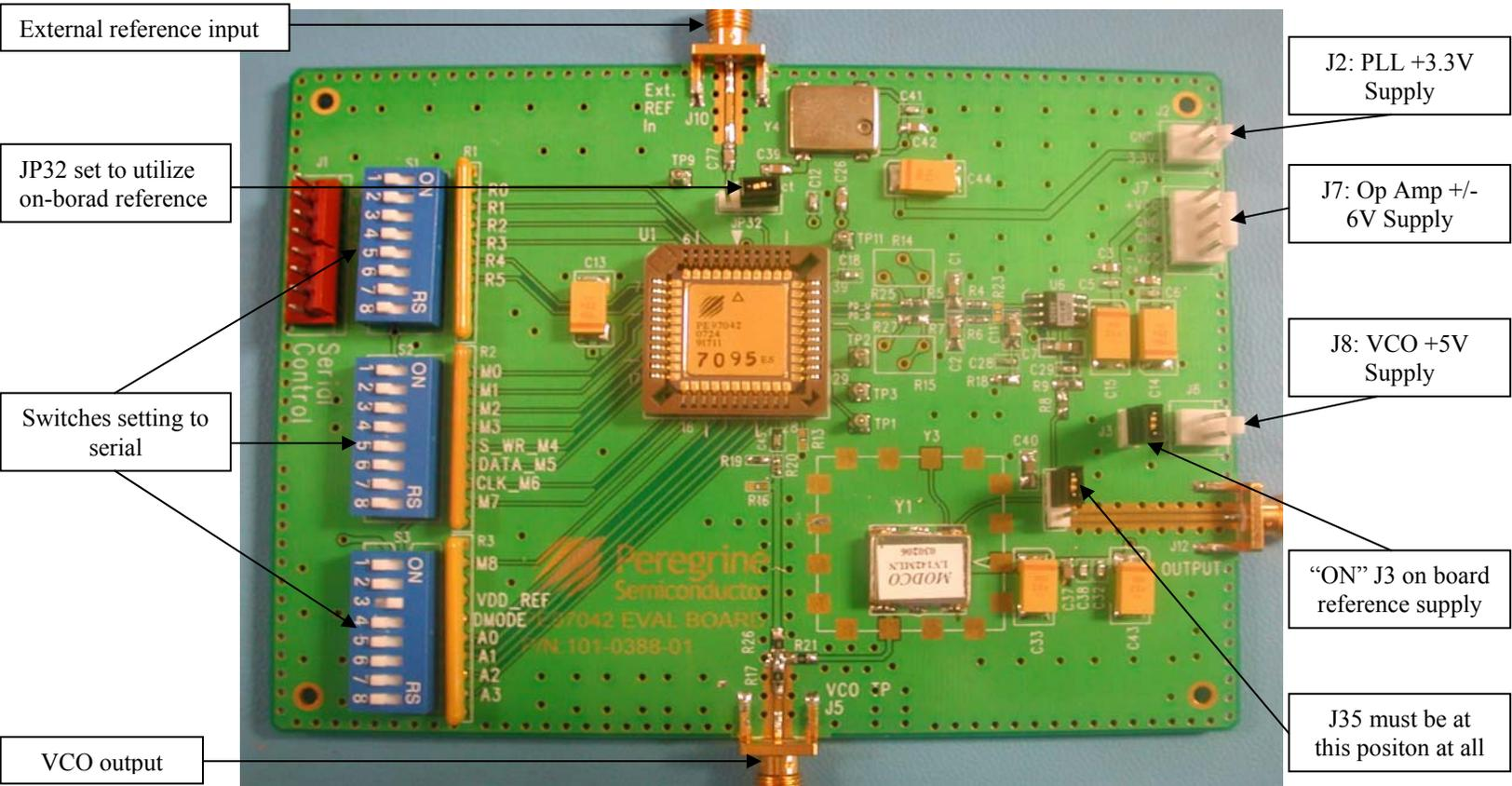
**Figure 3. Jumper Setting to Disable On-board Reference.**
