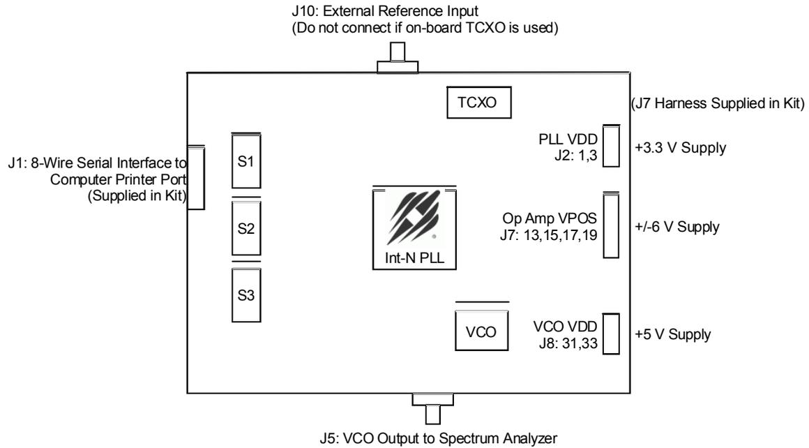
**Figure 2. Evaluation Kit Default Jumper & Switch Settings.**
