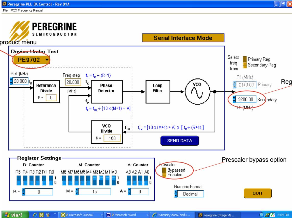
**Figure 4. PE97042 Software Control Panel**
