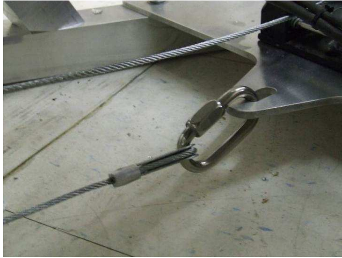
Figure 44 – Boom Winch Cable Termination
