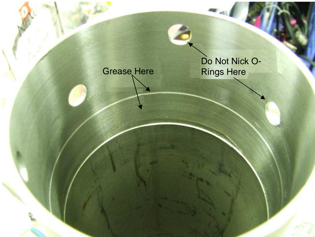
Figure 52 – Installing Pressure Sealing O-rings
