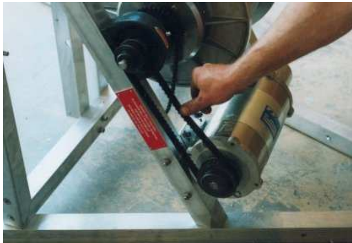
Figure 5 – Installing the Drive Belt
