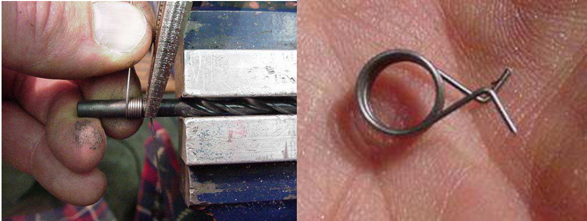
Figure 40 – Fabricating Core Dog Springs
