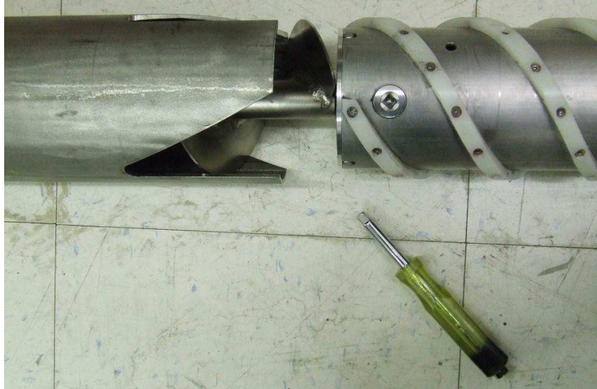
Figure 50 - Inserting the Short Barrel
