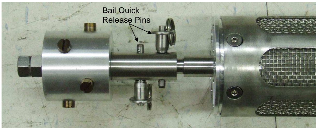
Figure 48 – Booster Pump Connection
