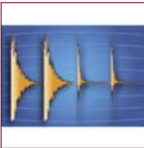
Fig. 2 Resonant ring-down reduction waveform & Dampened ring-down reduction waveform
