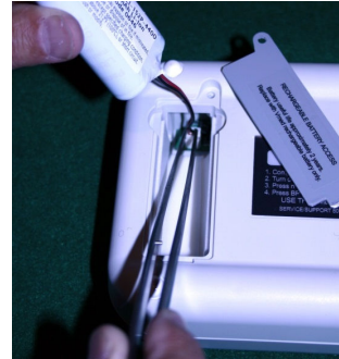
Figure 13 Use tweezers or forceps to place the plug of the replacement battery over the battery socket and press into place by pressing down on top of the plug. Place the battery into the compartment ensuring that wires are not pinched and replace the cover.
