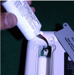
Figure 12 Remove cover from the back of the device and remove the battery from its compartment. Stretch the wires to their full length and pull the battery straight up to remove the battery plug.
