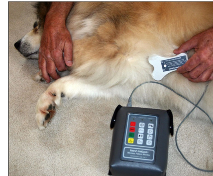
Figure 3 Correct position of the chest probe over heart on left chest oriented Right Front to Left Rear legs. Apply alcohol liberally for good signal.
