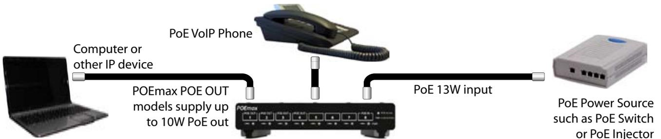
Figure 2 - POE<sub>max</sub> as PoE-Powered switch: connect POE<sub>max</sub> POE IN to a PoE switch/injector. POE<sub>max</sub> will operate as a network switch. POE OUT models can rebroadcast power to other PoE-Powered devices such as VoIP phones and IP cameras.
