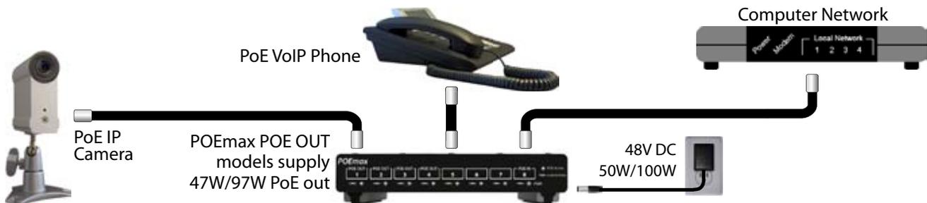
Figure 1 - POE<sub>max</sub> switch as PoE power source: connect POE<sub>max</sub> to power supply, computer network, and PoE powered devices such as wireless access points, VoIP phones, and IP cameras (NetMedia iViewHD).
