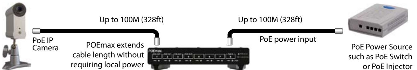
Figure 3 - POE<sub>max</sub> as PoE-Powered data/cable extension: connect POE<sub>max</sub> POE IN to PoE switch/injector. POE<sub>max</sub> will extend Ethernet cable length up to another 100M. POE OUT models can still redistribute any available PoE power.
