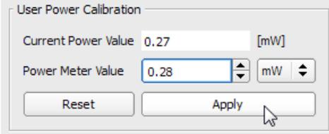
The image shows a dialog box titled "User Power Calibration". It contains two input fields: "Current Power Value" with a text box containing "0.27" and a unit selector "[mW]"; and "Power Meter Value" with a spin box containing "0.28" and a unit selector "mW". Below the fields are two buttons: "Reset" and "Apply". A mouse cursor is pointing at the "Apply" button.
