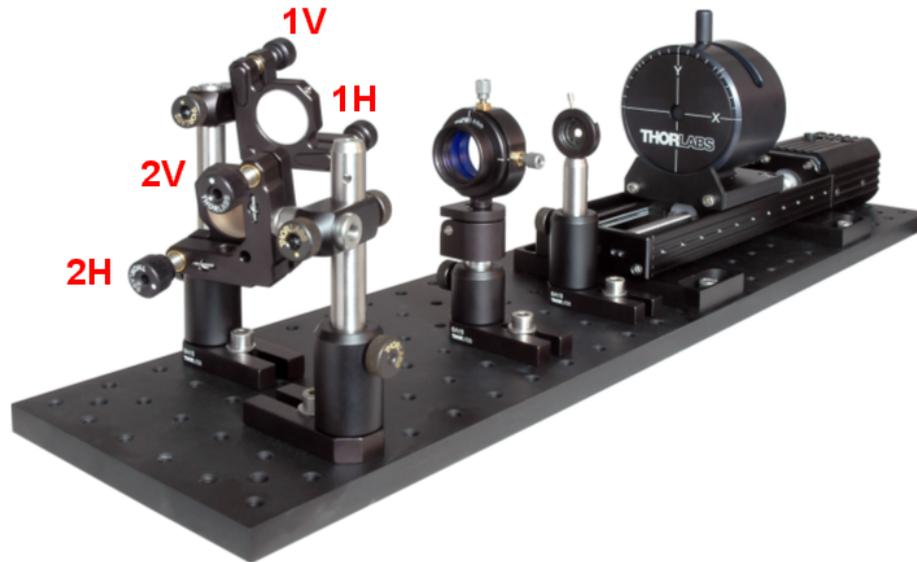
All beam quality parameters including  $M^2$  remain unchanged by this beam redirection using high quality mirrors.
