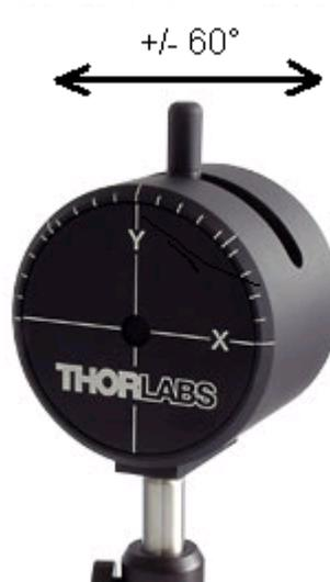
The rotation mount is essential for measurement the beam ellipticity, for instance. Since the major and minor axis of an elliptical beam may have arbitrary position in space, the scan axes of the Beam Profiler needs to be oriented to these axes in order to measure the real ellipticity.
