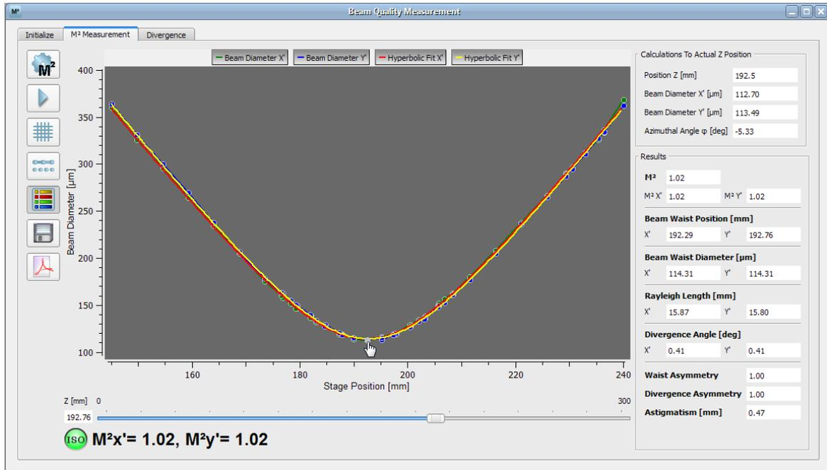
The green bulb indicates that the measurement was successful and fulfills the ISO 11146 standards.
