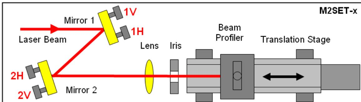
The beam is reflected successively at mirror 1 and mirror 2 in order to adapt beam height and align its direction towards the Beam Profiler. Adjustment screws of both mirrors are labeled within this figure according to its influence on the horizontal (**1H**, **2H**) or vertical (**1V**, **2V**) beam position and direction. These four adjustment screws are labeled also in the following photograph:
