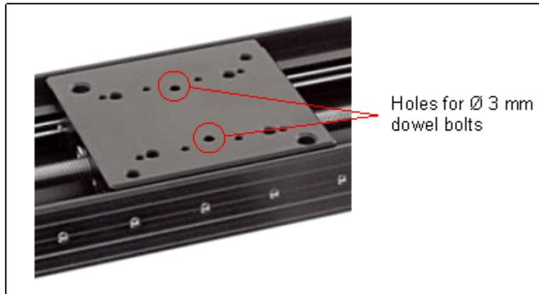
Put the adapter plate with the Beam Profiler mounted on it onto the mounting plate of the translation stage so that the two dowel bolts guarantee a nearly free from play connection. Fit both plates with 2 screws near the back plate of the Beam Profiler.
