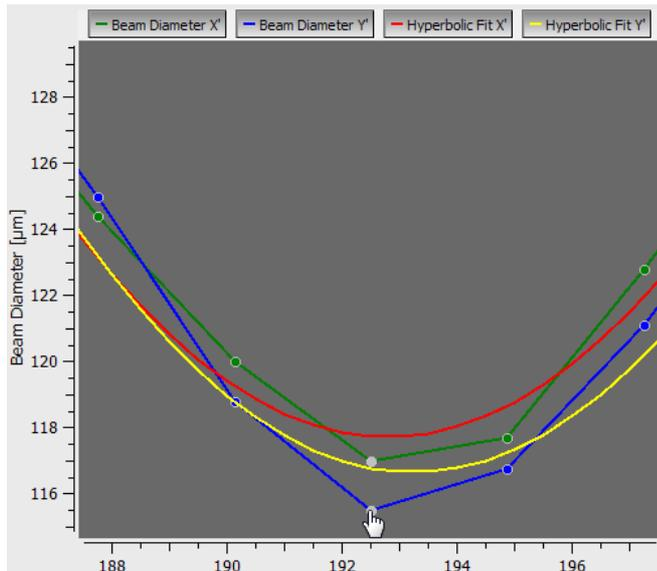
In above example, the fitted Y' beam diameter (yellow) is larger than the measured Y' diameter (blue); same is for X' diameters.
