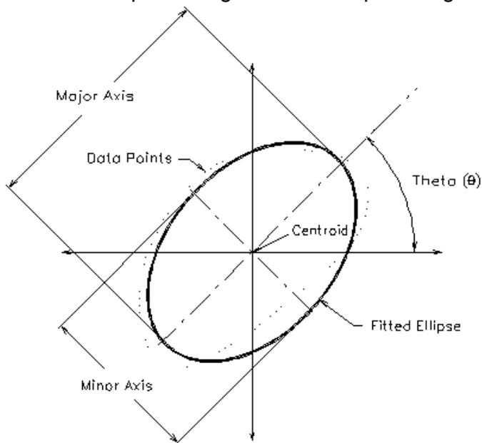
**Diameter (clip level)** is given for the minor axis (**min**), major axis (**max**) and their arithmetic **mean** value.
