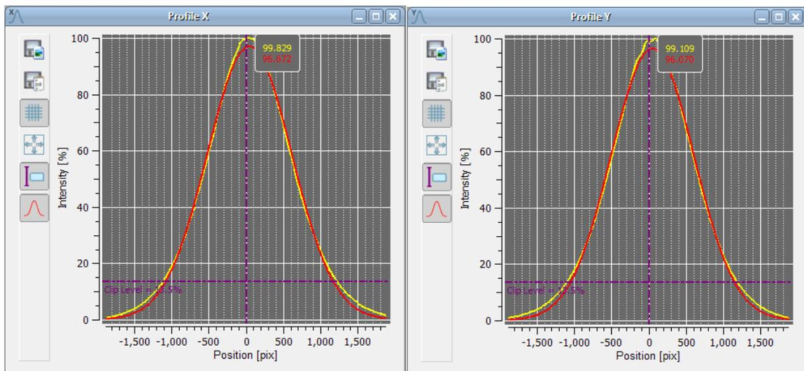
X and Y profiles display the intensity along the appropriate axes as marked on the front panel of the beam profiler.
