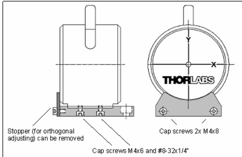
See [BP1M2 Mounting Adapter](#)<sup>[137]</sup> for a detailed drawing of the adapter. First mount the Beam Profiler onto the adapter plate by using the appropriate M4x6 and #8-32x1/4" screws, delivered with the BP1M2 Extension Set. Then push it slightly against the stop at the front. This guarantees orthogonal to the moving direction of the translation stage adjustment of the instrument. Then fix the screws.
