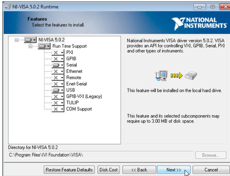
In this screen the required components are being selected. USB is required for the Beam Profiler control, Serial (RS232) for control of the translation stage used for M<sup>2</sup> measurements.
