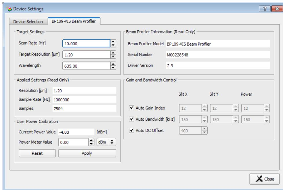
Make sure, the correct **Wavelength** is entered, and click "Close" to work immediately with the selected instrument. For details on Beam Profiler Settings, please see section [Device Settings](#)<sup>[46]</sup>.
