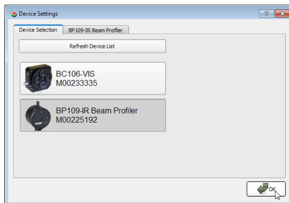
On panel 'Device Selection' choose a connected Beam Profiler instrument from the list and click 'OK' for its activation. Use 'Refresh Device List' to see also instruments very recently connected to your PC.
