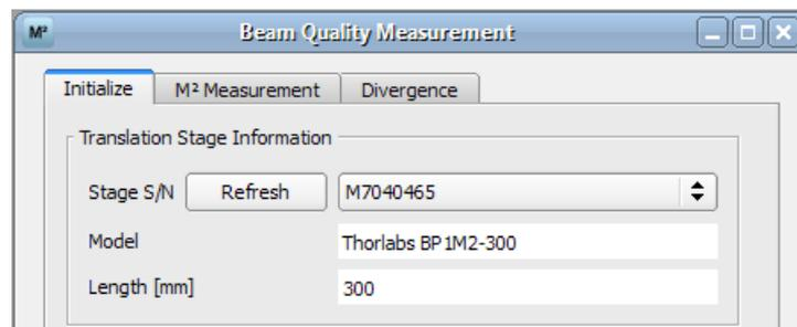
If connect the stage after starting software, it must be initialized manually.
