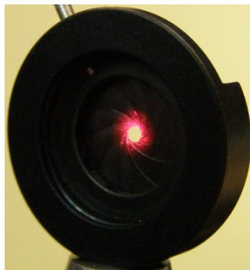
For infrared beams use a IR viewing card or alignment disk for visualization. In addition, the beam position is also displayed within the Beam Profiler software.
