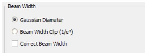
**Beam Width Clip (1/e<sup>2</sup>):** This is the value specified in ISO standard 11146. If a different clip level was used for normal Beam Profiler operation this will be overwritten by the M<sup>2</sup> measurement initialization.
