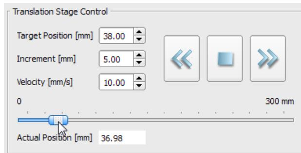
**Velocity** can be set between 1 and 13mm/s and remains valid for all subsequent operations. Default: 10mm/s.
