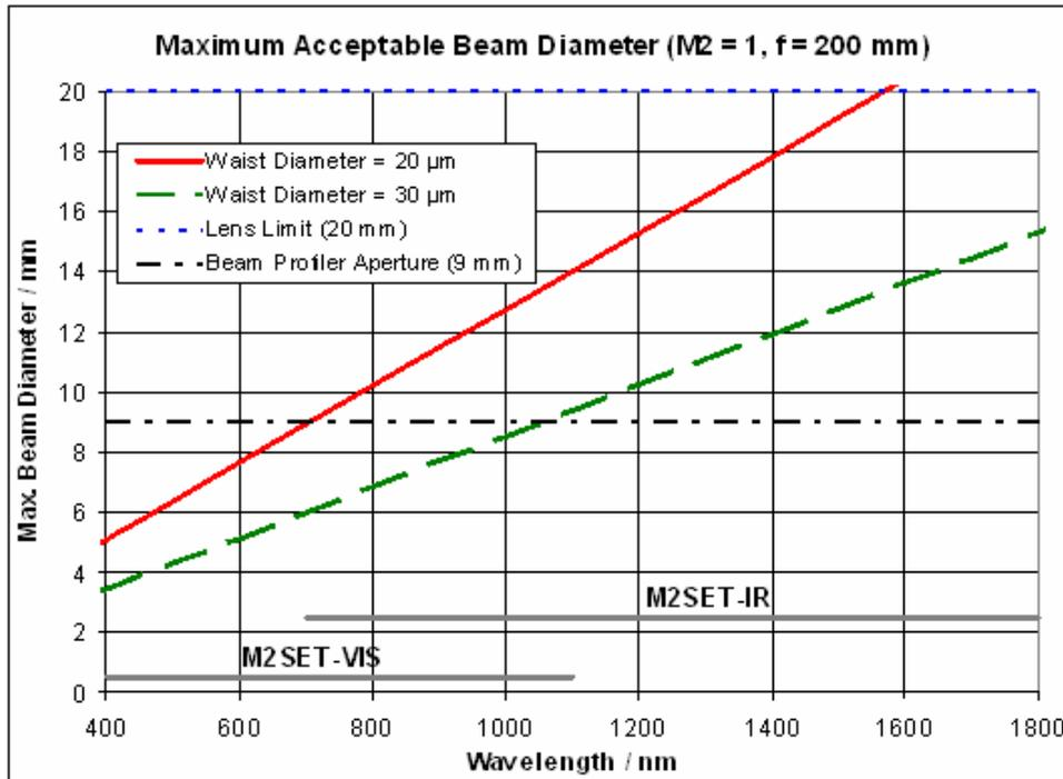
Select your operating wavelength at the x-axis and go up to the curve representing waist diameter. Then read out the max. acceptable initial beam diameter at the vertical axis. For a waist diameter at the measurement limit (20 μm, red curve) an operating wavelength of 633 nm yields a max. beam diameter of 8.1 mm, whereas for 1064 nm the diameter can reach up to about 13.6 mm.
