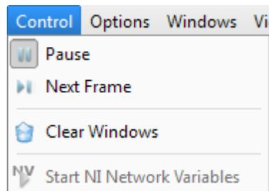
When the GUI is started or the active Beam Profiler instrument was changed, the application will start continuous operation automatically. Pausing the consecutive operation is advantageous for detailed analysis of a single image. User interactions will show increased performance on such a frozen image. The paused Beam Profiler can be restarted at any time.
