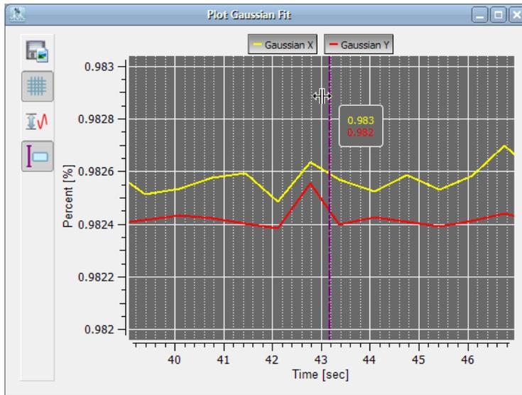
This window plots the Gaussian Intensity value (see [Calculation Results](#)<sup>34</sup>) which shows the coefficient of determination of the fit.
