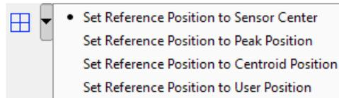
This displays the centered to the beam profiler's aperture crosshair. Together with the enabled **Centroid Cross** it's easy to observe beam centricity.
