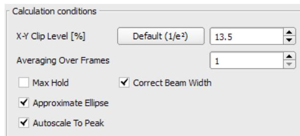
The **X-Y Clip Level** defines a relative intensity level between dark level (0%) and peak level (100%) of the measured beam profile used to measure the beam width,
