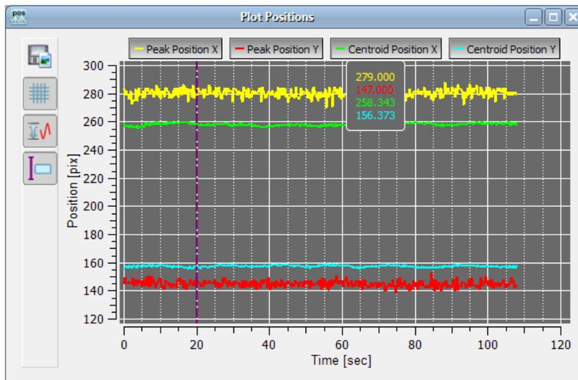
The positions of X and Y peak and of X and Y centroid positions can be displayed vs. time.
