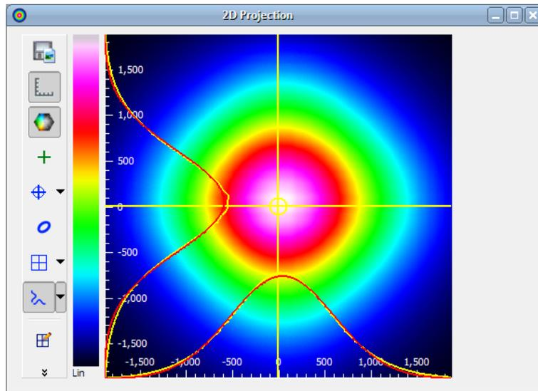
As the window name indicates the 2d image is based on a reconstruction since a slit beam profiler with two slits only provides two real cross section, i.e. x and y profile. The remaining pixel values are calculated by multiplying the normalized cross section values of the respective row and column. An additional bottom clipping is done for restraining amplified noise.
