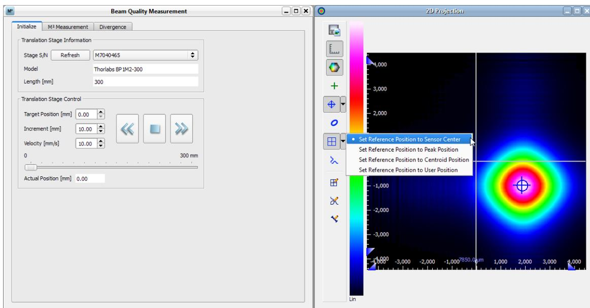
For beam alignment, the manual [Translation Stage Control](#)<sup>[85]</sup> is used, while the beam position is observed in the 2D Reconstruction panel. For more convenience, enable the Reference Position crosshair (set to sensor center) and enable the centroid cross.
