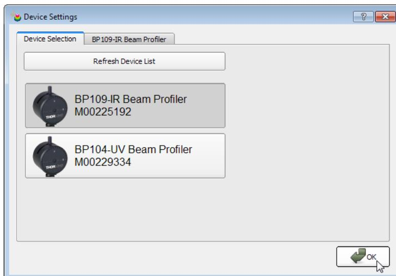
Usually the Beam Profiler connects automatically to the first connected camera. If you want to use another connected camera click onto an entry of the instrument to mark it and click 'OK'.
