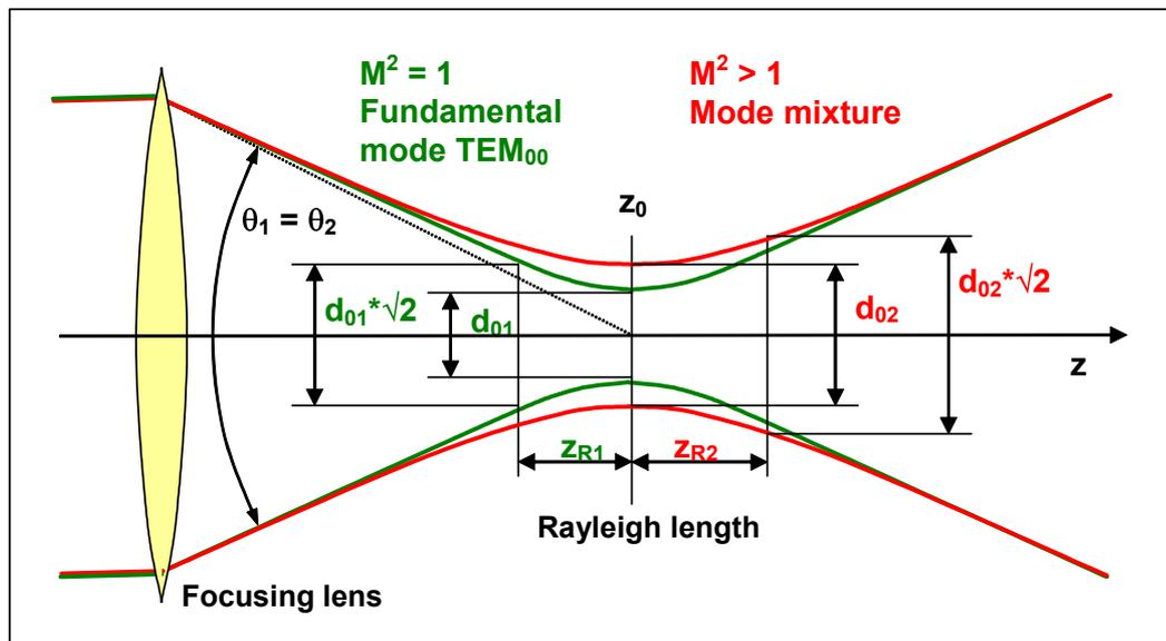
The Rayleigh length may also be influenced due to the changed beam propagation curve.
