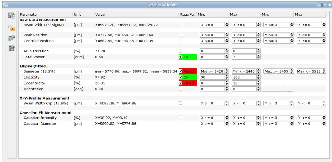
For each parameter a minimum and maximum can be set. Pass/Fail test result will be displayed only for those parameters, where the appropriate box in Pass/Fail column is checked. The test result status will be displayed beside the check box verbally and by red/green color.
