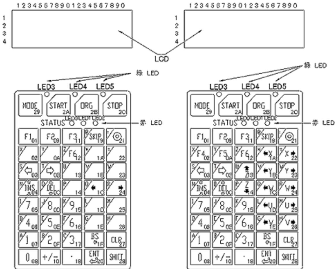
The hexadecimal values shown in bold face at the bottom right corner of each key represent the code to be sent out when the key is pressed. For example, if <F1> is pressed, *ProfiRT3* will send out “01” (hexadecimal). When <F1> is released, *ProfiRT3* sends out “80 + 01” (hexadecimal) by default.
