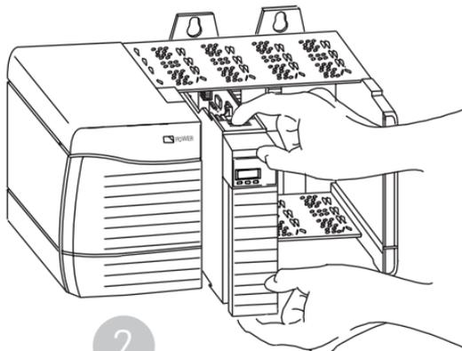
Slide the module out of the chassis.
