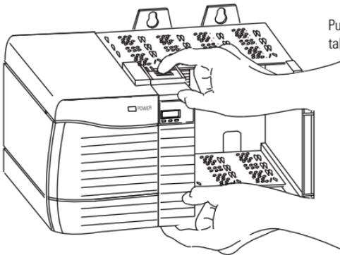
Push on upper and lower module tabs to disengage them.
