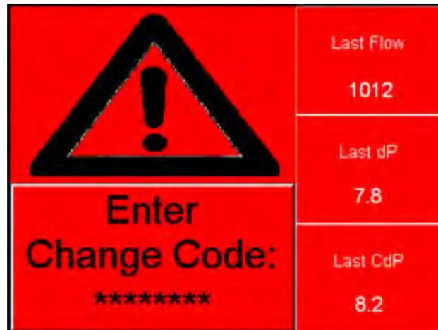
Example Flashing Critical Indicator
