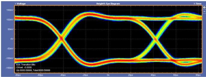
12 Gb/s 200 mV<sub>pp</sub> signal measured with a P7630 and a P76CA-292C coaxial adapter
