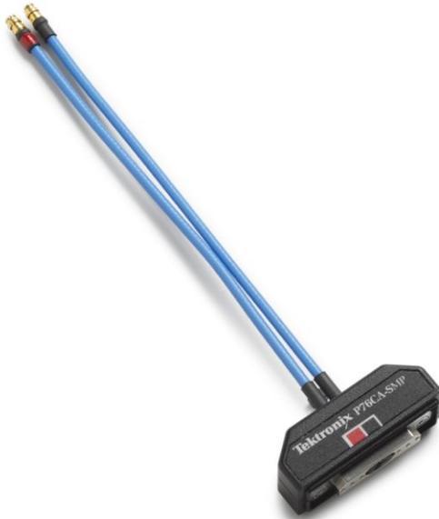
33 GHz Bandwidth Coaxial Adapter with SMP (Female) connectors and 6" of high performance cable. This adapter is calibrated at the input connectors and is ideal for directly connecting to devices with SMP output connectors.
