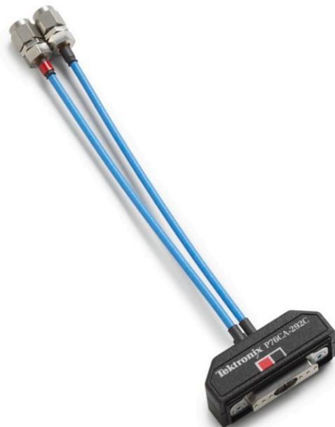
33 GHz Bandwidth Coaxial Adapter with 2.92 mm (Male) connectors and 6" of high performance cable. This adapter is calibrated at the input connectors and is ideal for directly connecting to devices with 2.92 mm or SMA output connectors.
