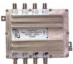
Hook up to a Bell dish with 2 dual LNBs to pick up 2 satellites at the same time, works with up to 4 receivers, zinc die cast housing, all port F-(f) connector, 75 ohm.
