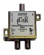
Enables you to receive satellite signals from two satellite locations to one Dish Network or Bell TV receiver. Combines two legacy dual LNBF's into one coax line. For a dual tuner receiver or 2 single tuner receivers, 2 of these are required. Bell TV (satellites 82 & 91) uses the SW21 switch to upgrade from SD to HD or international programming. Dish Network uses the SW21 switch for all SD (satellites 110 & 119) one and two receiver installations.
