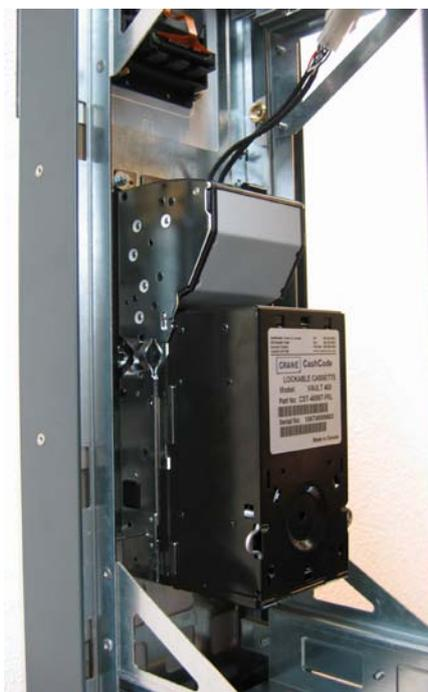
**Photo 7-4** The bank note acceptor with cash box module built into the MultiBank
