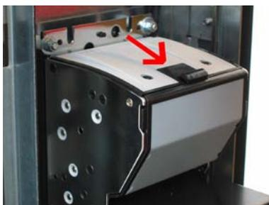
**Photo 8-2** Button for opening bank note reader
