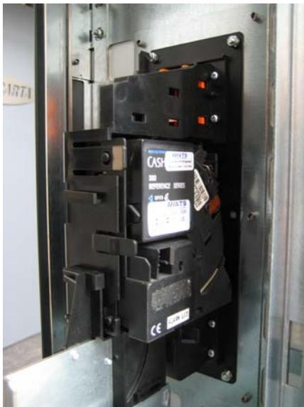
**Photo 7-1** Coin acceptor in transfer terminal
