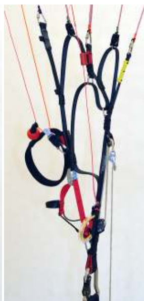
Pulley in first (highest) position with trimmer closed; EK magnet placed above the middle pulley position
