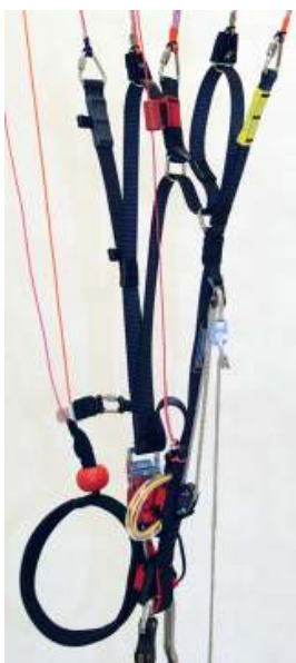
Pulley in third (lowest) position with trimmer closed; EK magnet placed above the trimmer buckle
