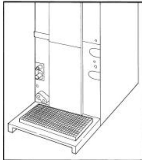
Fig. 5—Removing Filter from Fan Coil Unit
