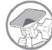
Notice by wipers cleaned area on the windscreen. Find a suitable location for the camera. Remove the protective strip from the adhesive foil and attach the bracket with the camera on 2.1 the windscreen or 2.2 inversely on the armature.
