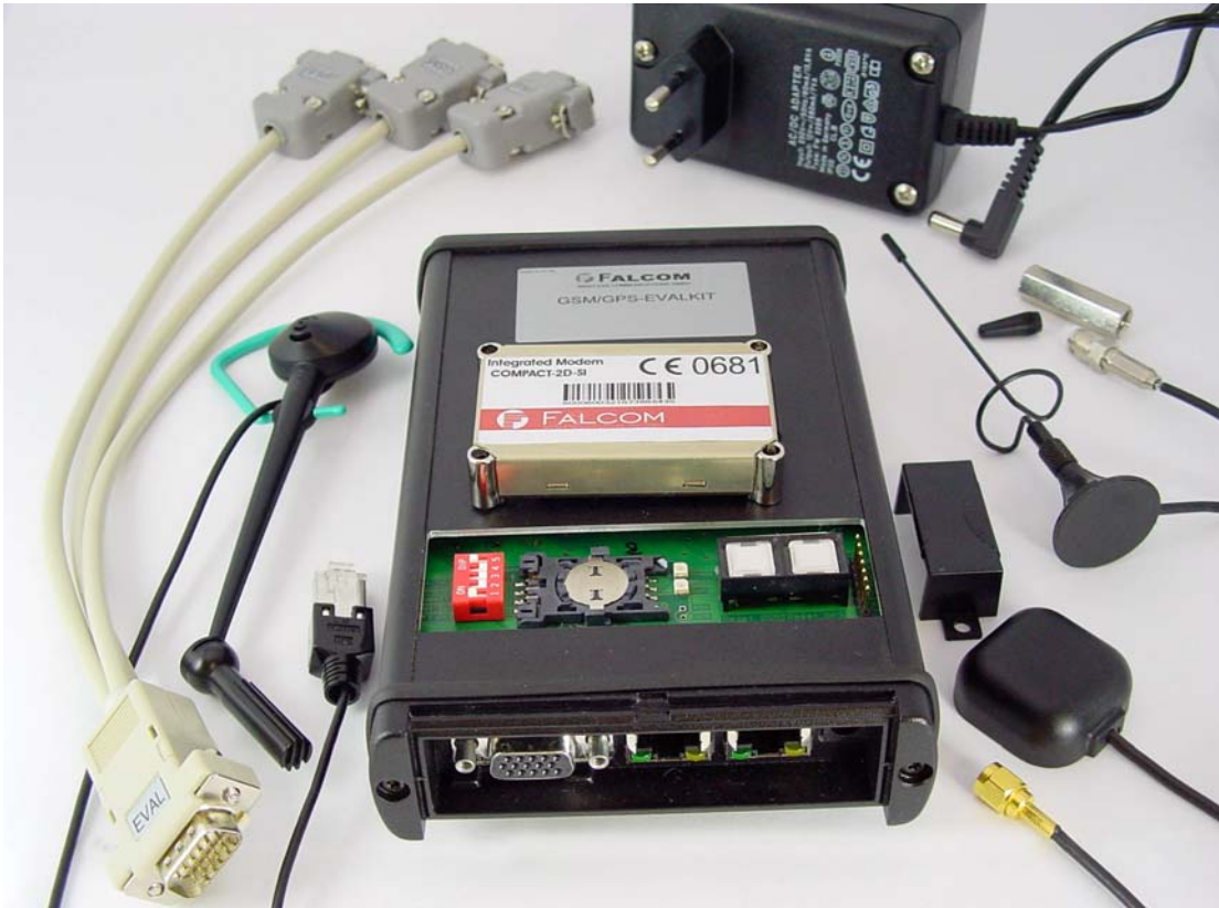
Figure 10: The FALCOM GSM/GPS evaluation board (EVAL-KIT)
