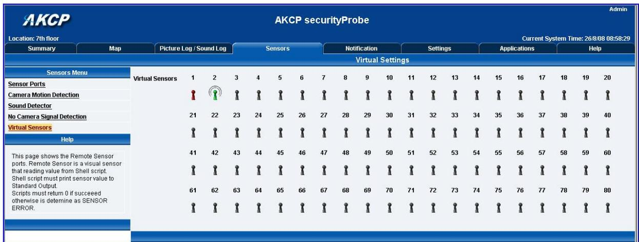
Click on the first available virtual sensor (in this case 3) you can then choose what type of sensor to setup from the next screen. First click on the “**Configuration**” button, then you will have a choice of SNMP Get, Ping, Custom Script, MODBUS, Boolean, or Trap Receiver.
