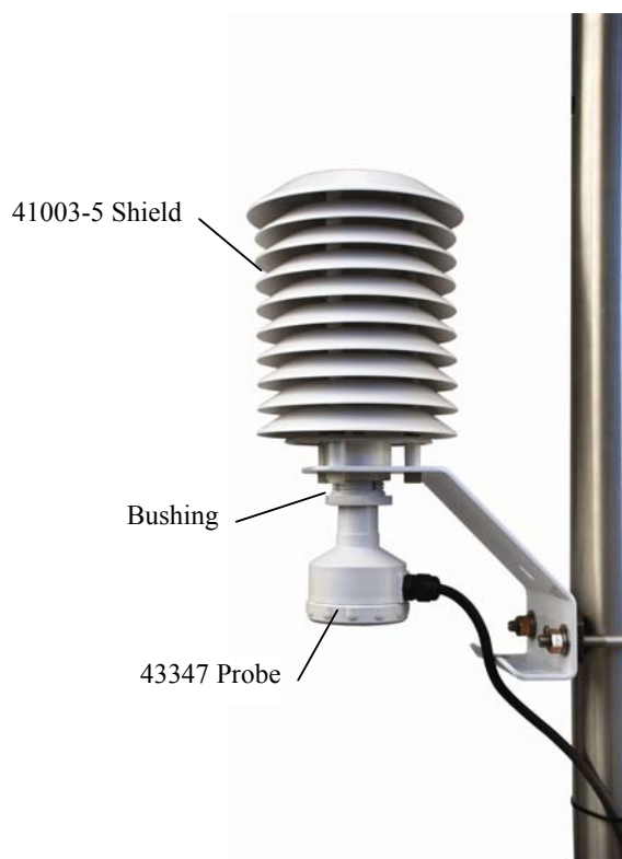
Figure 3-3. 41003-5 Radiation Shield Mounted to Tripod Mast
