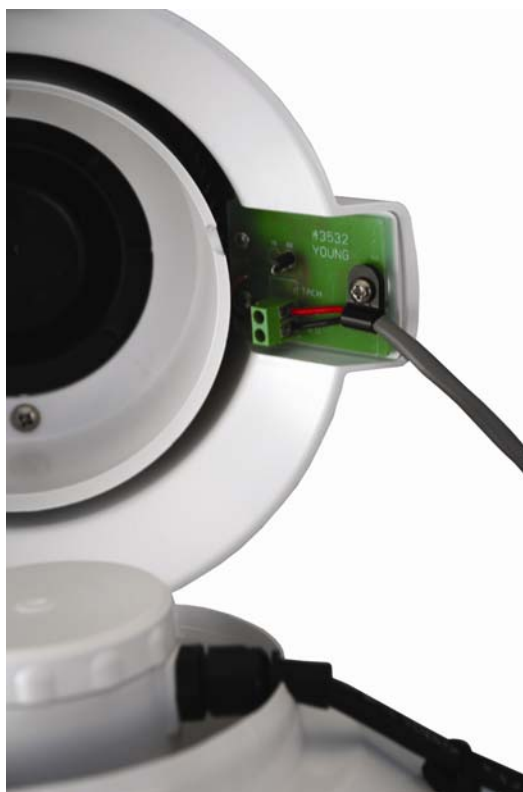
Figure B-2. 43502 Shield Power Connections
