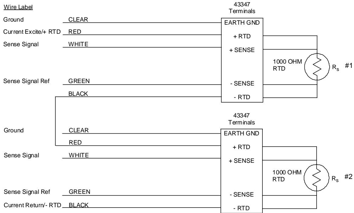
Figure D-1. Schematic for Two 43347-IX Temperature Probes
