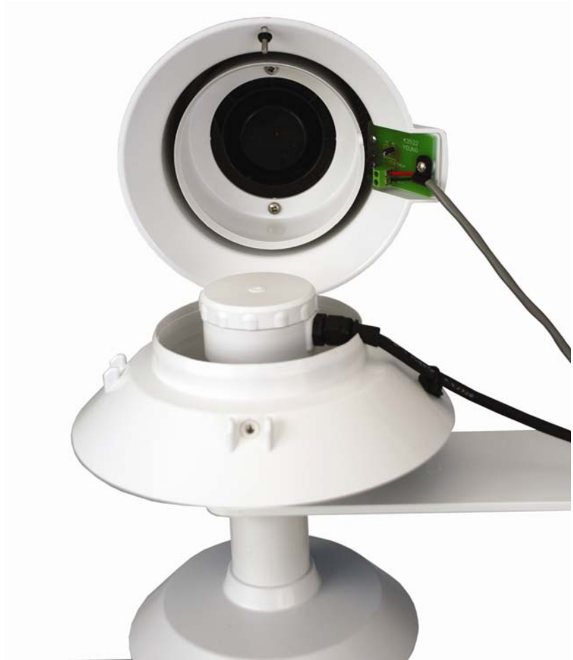
Figure B-3. 43347 Probe Mounted Inside the 43502 Shield
