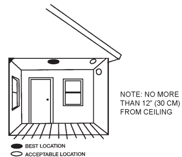
FIGURE 5: RECOMMENDED SMOKE ALARM MOUNTING LOCATIONS.
